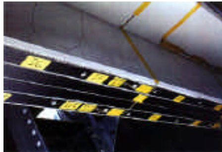
Fig 5 B1-Beam before Fatigue test
